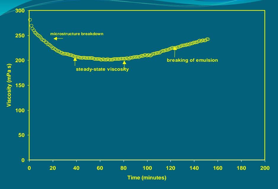
CRS-2 Equilibrium Viscosity at 50, 100, 200 RPM and 50 °C, Spindle #21
