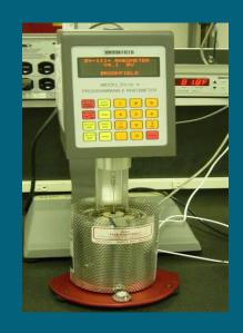
ASTM D 7226 viscosity by rotational Paddle viscometer (2006 to present)
