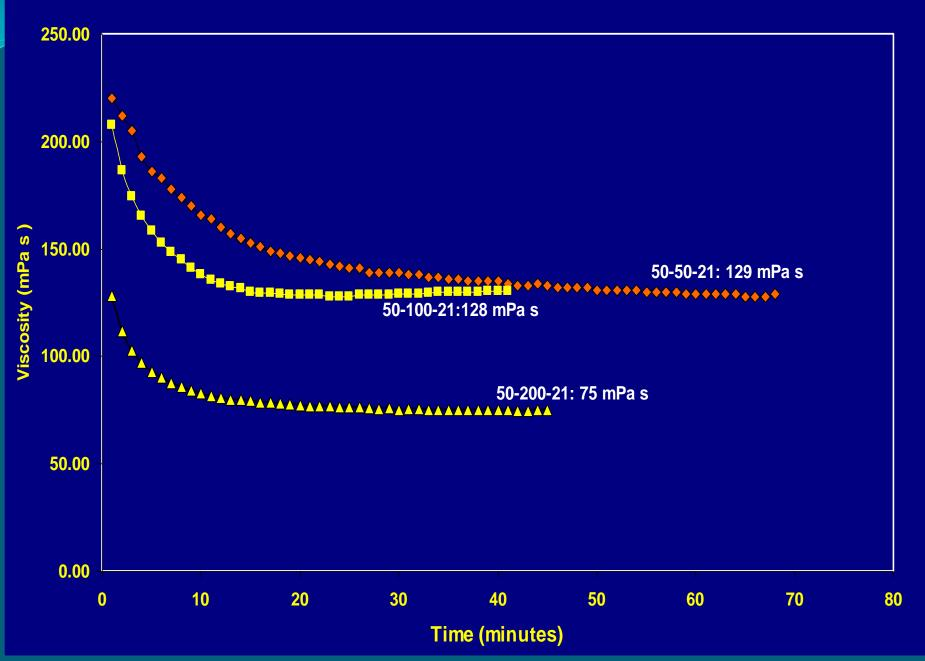
CRS-2 Equilibrium Viscosity at 50, 100, 200 RPM and 50 °C, Spindle #21
